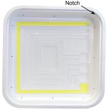
Unpack the incubator from the box. Remove the top half from the bottom. Lay the **Plastic Liner** in **Hova-Bator Bottom** then place the **Incubator Floor** on top of the **Liner**. Arrange the plastic floor as shown using the water troughs and turner power cord notch as reference. In most climates, fill trough #1 (highlighted in yellow) with water. Surface area, not depth, determines humidity; refill trough as necessary to prevent it from drying out.
