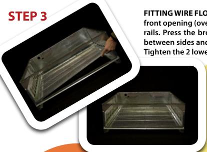
FITTING WIRE FLOOR IN BROODER - Insert the wire floor in through the front opening (over the top of part #4) and down into drop pan support rails. Press the brooder sides in or out to leave about 1/16" clearance between sides and the wire floor.
