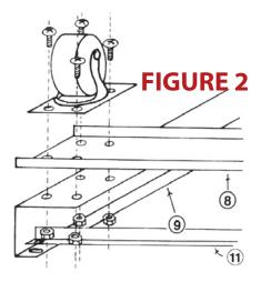
MOUNTING PLUG STRIP TO BROODER (#10) - Remove bolt "A" (Figure 1) from back left corner of brooder. On the back of the Plug Strip are 2 bolts with 2 nuts on each bolt. Remove one nut from each bolt on the plug strip. Insert the bolts on the plug strip into holes "A" and "B", Figure 1. Put the 2 nuts that were removed, back onto the bolts and tighten them. When used on a Battery, the Plug Strip should be mounted on the second or third brooder, so all electric plugs can reach the Plug Strip.
