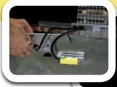
**HEATER SUPPORT** - Attach Heater (#6) inside the aluminum channel (#7)
