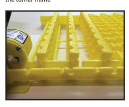
**3.** Line the egg racks up with the correct slot in the connecting bar. Starting at one end, press firmly to snap the rack into the connecting bar
