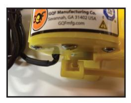
**4.** Once all racks are snapped firmly into the connecting bar, line the connecting bar (slot) up with the (white) swing arm on the turner motor. Press the connecting bar firmly so that it "snaps" onto the (white) swing arm of the turner motor.
